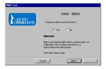
Select Yes and then click on Next to start the procedure. Immediately following the Zero procedure, a Calibration Certificate is opened.
