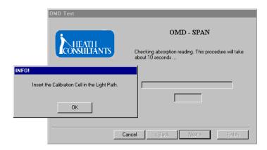
Place the external Calibration Cell into the light path by attaching it to the receiver's mounting studs and click OK. After span calibration is complete, the certificate data is again collected. You can print out the report and use it as a reference or just close the Calibration Certificate window.
