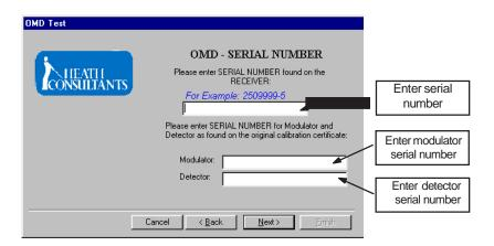
Once the modulator and detector serial numbers are input, it is not necessary to re-enter them to use the program for the same OMD. Only the receiver serial number will be required. New or different serial numbers resulting from repairs or upgrades will need to be re-input, but only to update the database and only input once.
