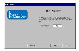
The TSP Adjust procedure will start by increasing the TSP by  $+0.1^{\circ}$  C. Wait 3 minutes for the temperature to stabilize.
