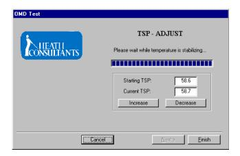
After stabilization, again note the PPM and Methane readings. If the PPM value became smaller and the Methane value became closer to negative Offset value, then the temperature change is in the right direction (Increase). If the values worsen, the temperature change is in the wrong direction and Decrease should be chosen. Should the values be acceptable (PPM zero within +/- 2), click Finish to accept the new TSP and generate a Calibration Certificate.
