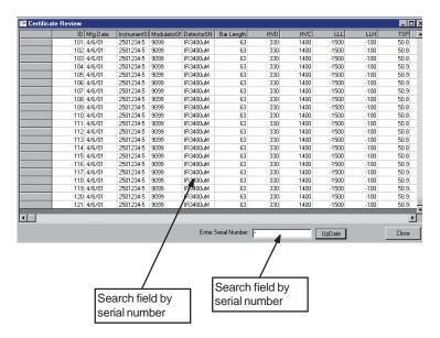
To view and print out the certificate, double click on the row of the certificate you want to print and the OMD Calibration Certificate will be shown in a separate window.
