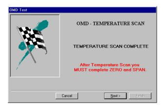
**Attn:** After Finish a window will pop up that says, "Now Allowing 10 minutes for stabilization". After that an Ok or Next button is highlighted. Click that and then 'Zero' and 'Span'. A calibration report will be generated automatically after each 'Zero' and 'Span'.
