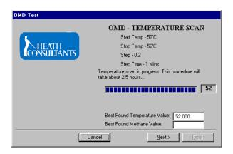
After the Temp Scan, both the ZERO and SPAN procedures will automatically be selected later. Click Finish to continue.
