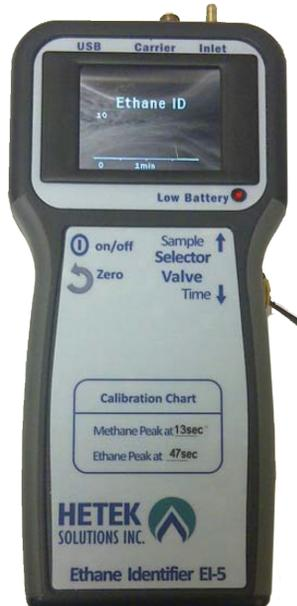
The Heath EI-5 Ethane Identifier is a portable combustible gas analyzer designed to differentiate between gas distributed by a utility and naturally occurring gas often present in the ground or sub-surface structures.
