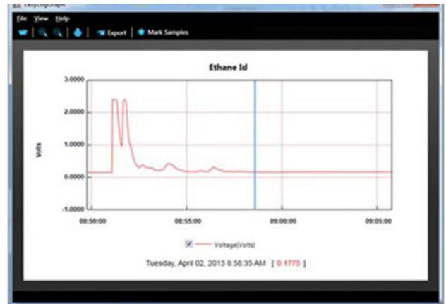
The data, when downloaded using Easylog software, is displayed in graphical form showing the peak(s) for the different gases in the sample taken. The sample above shows a typical natural gas sample indicating the date and time for each data point.
