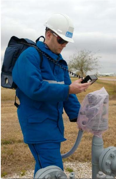
Whether you're managing a leak detection and repair program or active in greenhouse gas trading, the Hi Flow Sampler allows an accurate emission or leak rate to be made in less than one tenth the time required to perform an enclosure measurement. This portable, intrinsically safe,
