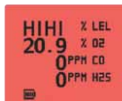
Red display in alarm conditions
