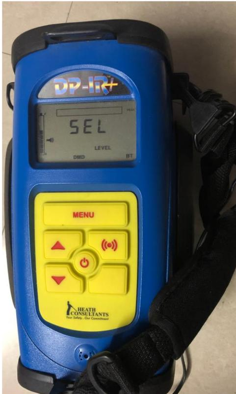
The Bar Hole Mode enhances a technician's ability to perform bar hole surveys by automatically controlling the pump while capturing the peak and sustained methane readings over a 15 second duration. Upon switching to the Bar Hole Mode screen, the DP-IR+ Pump should turn off.
