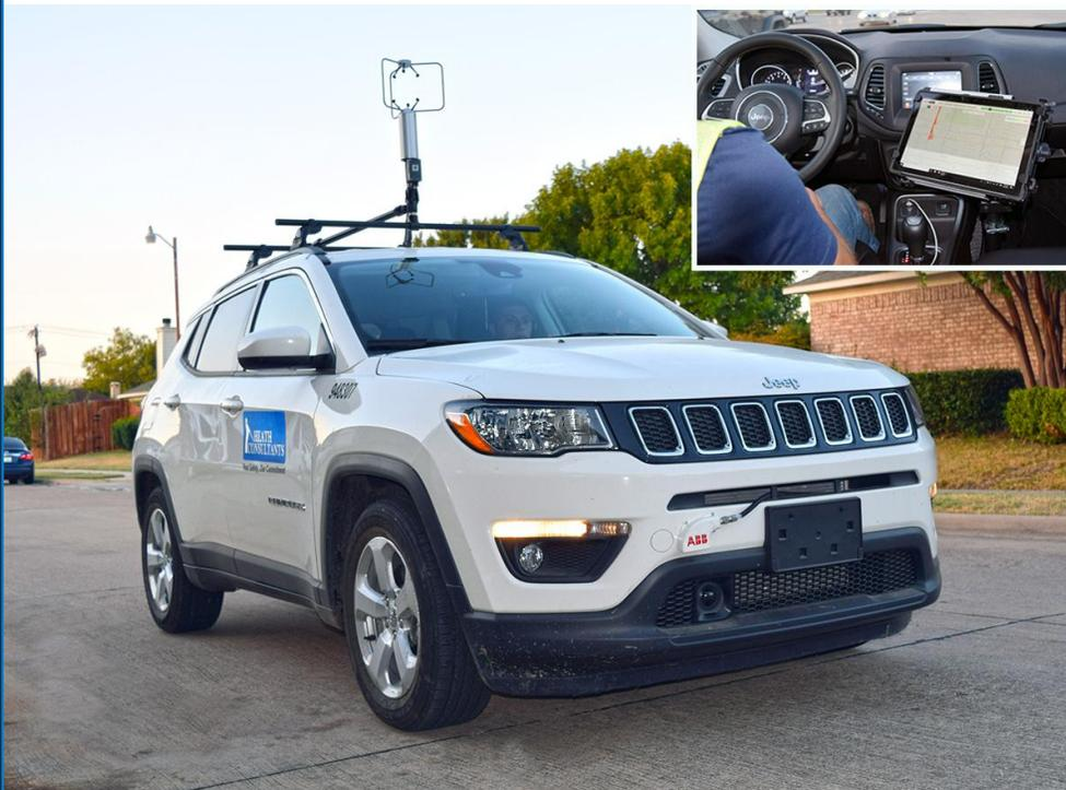
MobileGuard™ finds gas leaks quickly and efficiently with both real-time plotting of indications and gas discrimination as well as GIS integration capabilities.
