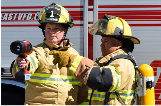
The RMLD-FR™ allows first personnel to quickly scan common venting points within a structure from a safe distance to determine if there's natural gas (methane) present. This instrument is based upon our highly successful RMLD legacy and RMLD-CS designs with many of the same features and
