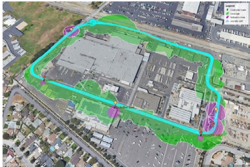
Survey route (turquoise), coverage area (green) leak indications (purple)
